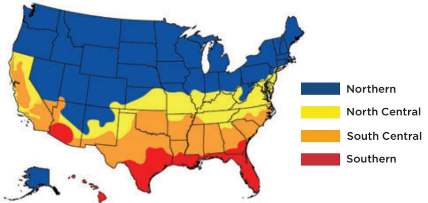
**Figure 3.** Builders can turn to the Energy Star program for help selecting the best windows for their climate. In northern regions, windows must be good at keeping in wintertime heat; in the south, they should be able keep heat out in the summer. Windows installed in the middle of the country must balance summer and winter performance. Note that all values in the table are based on NFRC whole-window ratings.
