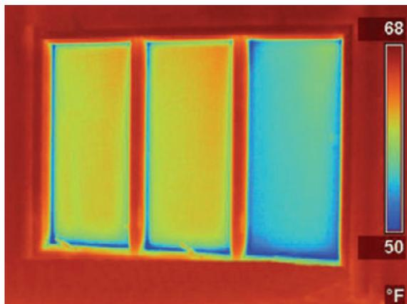
**Figure 4.** The inside surface of the low-E windows (left and center panes) are much warmer than that of the clear double-pane (right pane). If this window had three bays of clear double-pane glass, the room's heating thermostat would have to be 2°F to 3°F warmer to provide the same level of comfort achieved with low-E glass.
