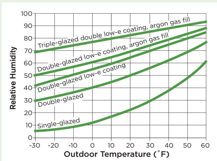
Given an outdoor temperature of 20°F, project up vertically to the desired glazing curve. A double-glazed clear window, for instance, corresponds to a relative humidity of 51 percent. Compare this with a double-glazed low-E argon product, which would allow almost 70 percent relative humidity before condensation would occur. This chart is for the glass only and not the frame.
