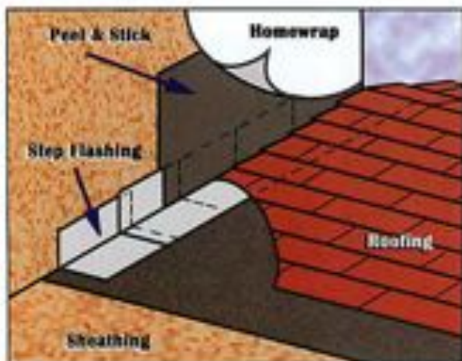
Photo 15 - Peel-and-stick flashing from sheathing onto metal flashing.
